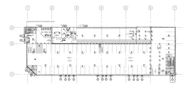
the facility. At the main entrance, lighting is controlled by a "reverse photosensor" that provides 80% light levels during daytime and 20% output during evening hours. Fixtures on all parking tiers and ramps are set to 20% output, increasing to 80% when motion is detected. In the stairwells and elevator lobbies, the fixtures are set to 20% output, increasing to full output when occupancy is detected.
