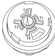
View of Z10 0-10V Device Receptacle
