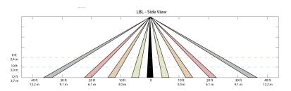
Note: The application/absolute range of the sensor is subject to variation because of different types of clothing, backgrounds, and ambient temperature. Therefore, ensure *that* the lens is properly oriented along routes with expected traffic and conduct testing along those routes.
