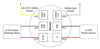
Note: If using a power pack other than PSC-AC-PP-200, connect either Control Hi or Control Low, depending on power pack relay circuitry.
