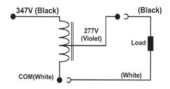
\*Lead Type: (AVLV2), Type 3321, No. 18 AWG (or Equivalent), rated 150°C, 600 V. Strip 10mm Tin Plated.
