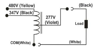
\*Lead Type: (AVLV2), Type 3321, No. 18 AWG (or Equivalent), rated 150°C, 600 V. Strip 10mm Tin Plated. 347V lead wire is pre-insulated.
