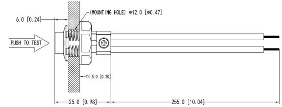
Dimension unit: mm [inch] / Tolerance: ±1[0.04]
