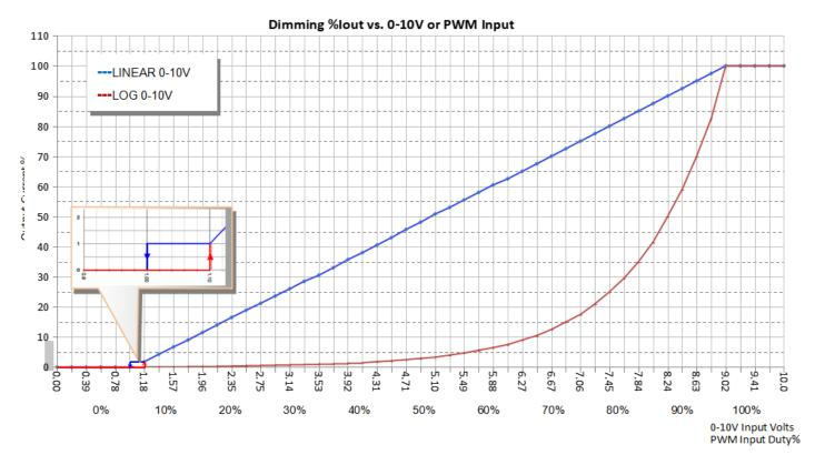
0-10V Dimming Curve @ Minimum dimming set to 10% and dim to off :
