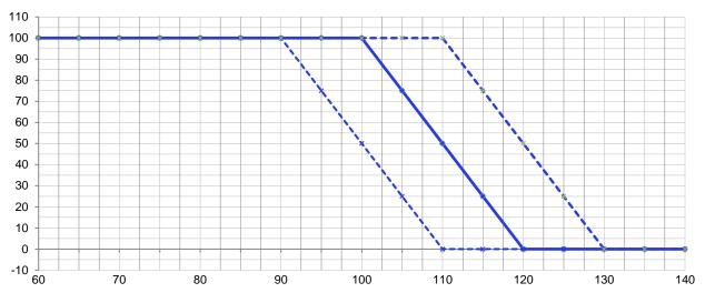
**Output Current% derating curve vs. TC Temperature**
