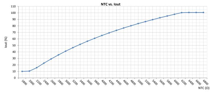
Note: Maximum dimming current is limited by NTC.
