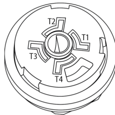
View of Z10 0-10V Device Receptacle
